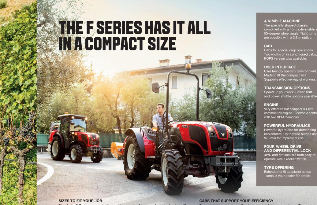
combined with a front axle enable a 55-degree wheel angle. Tight turns are possible with a 3.6 m radius.
